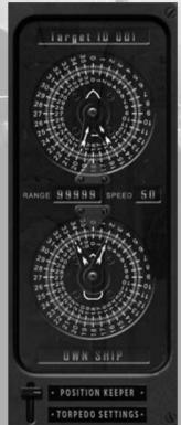
The great advantage that U.S. torpedo data computers have over those of other nations is the Position Keeper (PK). This unique device estimates the target data based on the initial values entered by the user. It computes the target movement in relation to your submarine, taking into account your own ship movements.
